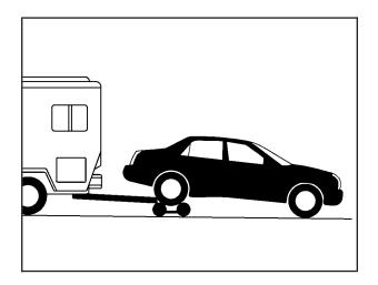
If you have a Rear-Wheel Drive (RWD) vehicle, it can be towed using a dolly. If you have an All-Wheel-Drive (AWD) vehicle, it can only be towed on a flat-bed trailer. To tow your RWD vehicle using a dolly, follow these steps:
